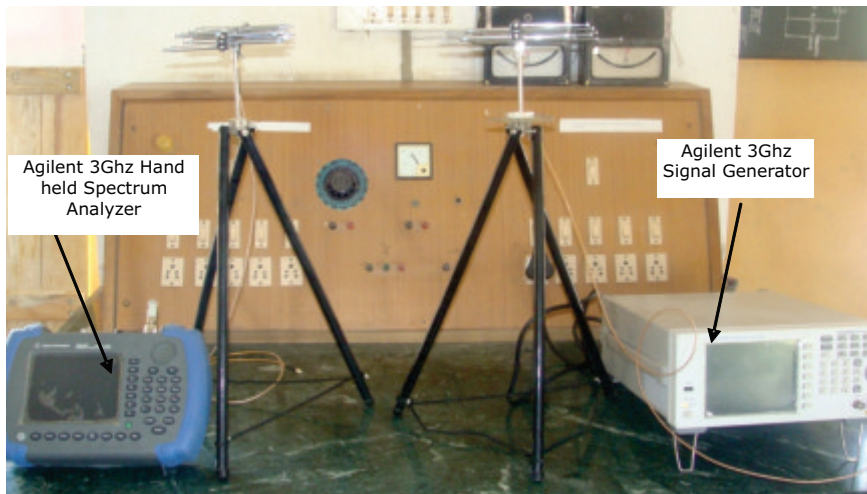
Figure 2. Overview of hardware used for propagation investigation.
